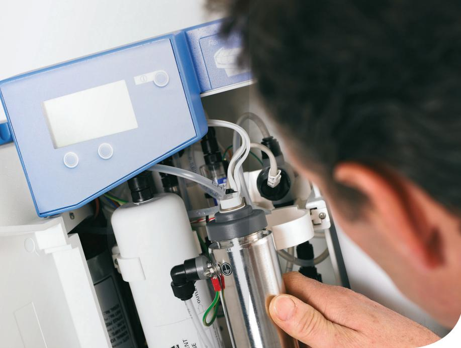
Carbon is used as either granules or molded and encapsulated cartridges, which produce fewer fine particles. Activated carbon reacts chemically with 2-4 times its weight of chlorine, and very rapidly produces chlorides; therefore even small carbon filters can effectively remove chlorine from water.
