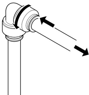
Unscrew connector and depress collet to detach tube
