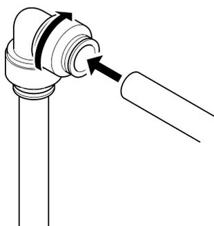
Push in tube and tighten connector to secure
