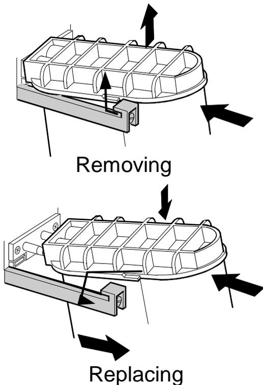
Purification Cartridge (LC207) and Conditioning Cartridge (LC206) removal and replacement.
