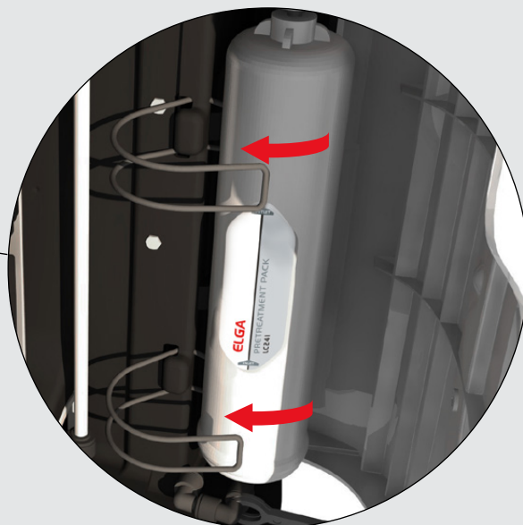
2. Change Pre-treatment cartridge LC241. (Optional)
